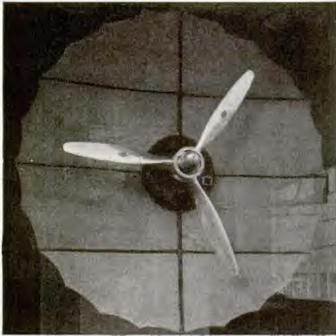
The wire mesh back of this propeller reveals errors in balance by fluttering; if it's perfect the mesh does not move
